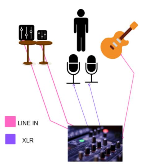
$\circ$  2/3 XLR (microphones).  $\circ$  1 Line IN for guitar.  $\circ$  2 mono/ 1 Stereo Line IN for analog synth. 2 mono/1 stereo line IN for sampler.
